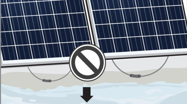
The illustration shows two solar panels mounted on a surface. Below the panels, a water level is indicated. A warning sign (a circle with a diagonal line) is placed over the water level, with an arrow pointing down to it, indicating that the connections should not be submerged.
